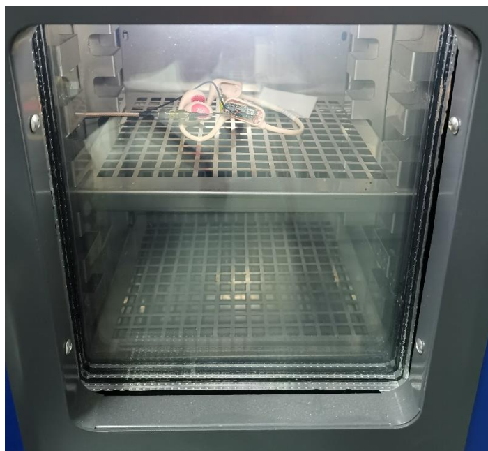
Photograph 2: Set-up for Radio Spectrum Testing, Extreme Condition
